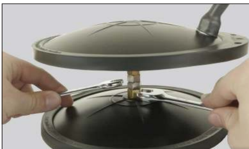
10. Use two 9/16" wrenches to tighten the jam nut
