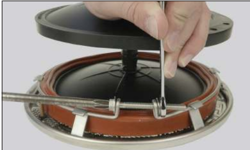
1. Use a screwdriver and a 7/16" wrench to loosen the wire clamp
