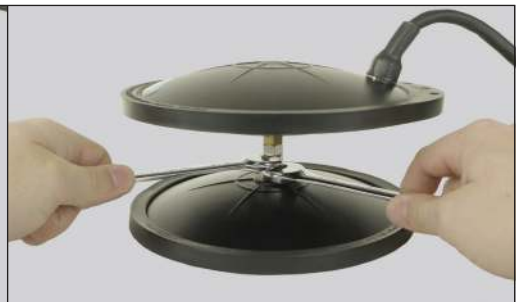
6. Use two 9/16" wrenches to loosen the jam nut
