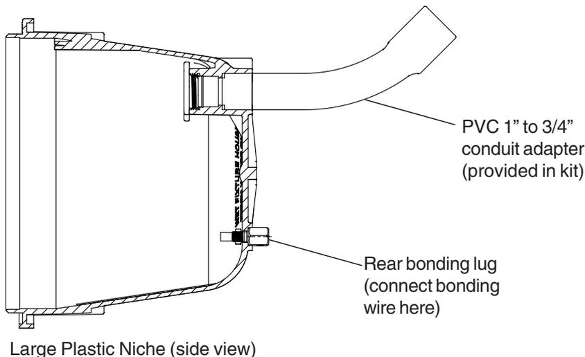
6. Support conduit to hold the Large Plastic Niche at the proper distance in front of rebar so that the front of mounting ring is flush with the desired finish surface.
