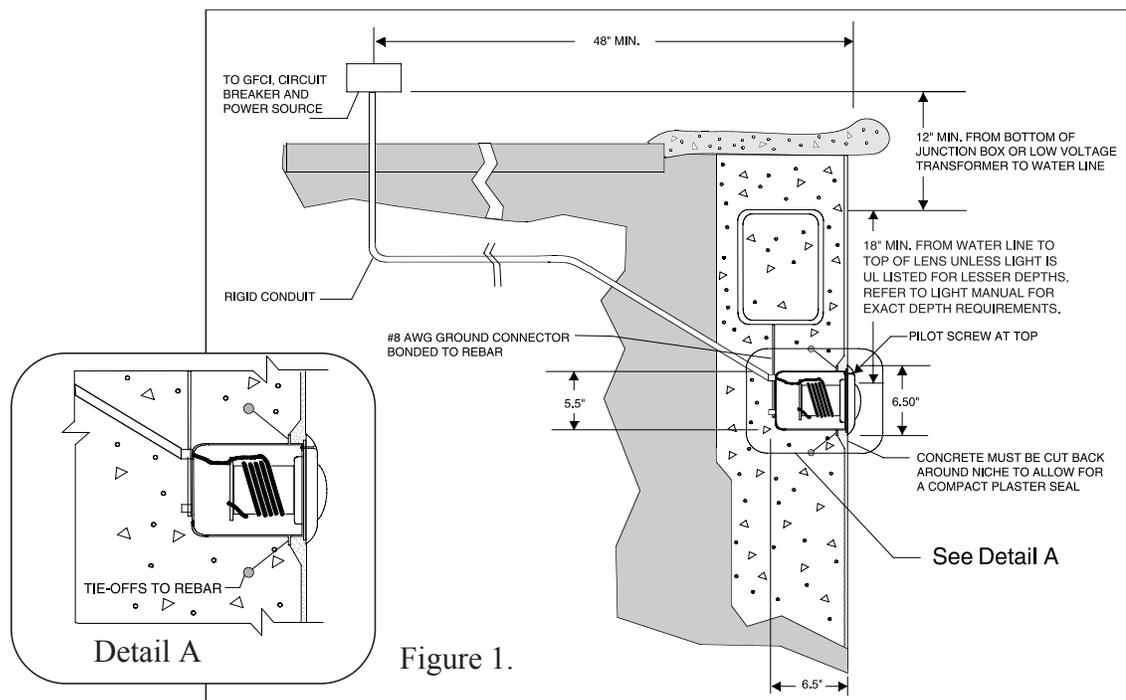
The niche is properly electrically bonded and grounded using the NO. 8 AWG ground connector located at the rear of the niche, see Figure 1.
