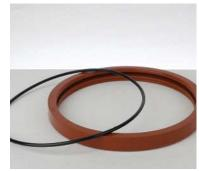
Install the mounting gasket around the rubber ring of the sound lens. The gasket's flat side will go towards the face ring. The grooved side faces the speaker body. Ensure the mounting gasket is installed evenly and is firmly seated against the entire circumference of the sound lens.
