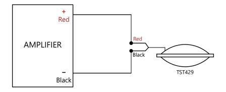
Clark Synthesis recommends an amplifier rated 125-150 Watts per channel at 4 ohms
