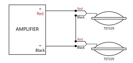
Clark Synthesis recommends an amplifier rated 125-150 Watts at 8 ohms
