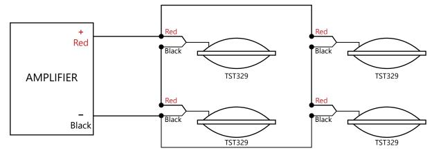
Clark Synthesis recommends an amplifier rated 500-600 Watts per channel at 4 ohms
