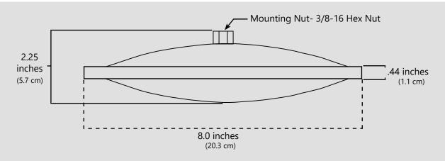
**TST329 Specifications:** • Continuous power handling: 135 watts • Impedance: 4 ohms • Overload Protection: Polyswitch • Frequency Response: 10Hz to 17kHz • Electrical Connection: 3ft. - 16/2 wire Dimensions: 8 in. diam. x 2.25 in. high • Recommended Amplification: 125 - 150watts at 4 ohms **Storage Temperature:** -148°F (-100°C) to 212°F (100°C)
