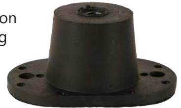
The entry-level TI-100 Isolation Foot is constructed of natural rubber and can be used as a low-profile foot replacement. Use of the TI-100 helps reduce vibration transmission into the floor and improves the performance of Clark Synthesis Transducers.
