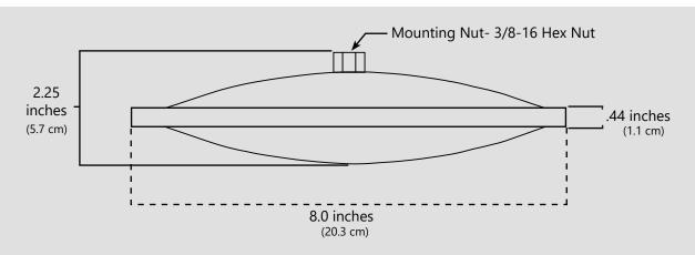
**AW339 Specifications**: • Continuous power handling: 135 watts • Impedance: 4 ohms • Overload Protection: Polyswitch • Frequency Response: 10Hz to 17kHz • Electrical Connection: 3ft. - 16/2 wire • Dimensions: 8 in. diam. x 2.25 in. high • Recommended Amplification: 125 - 150 watts at 4 ohms **Storage Temperature**: -148°F (-100°C) to 212°F (100°C)
