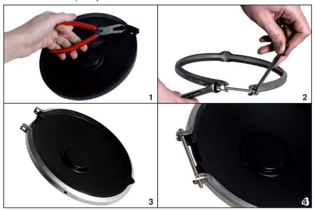
Carefully place the Hayward face rim (chrome side down) on a non-abrasive surface, and place the speaker and assembly clamp on the Hayward face rim (#5). Align the assembly clamp screw so that it does not cover the mounting tab or the face rim lockscrew. Once aligned, tighten the assembly clamp screw until the speaker is securely attached to the face rim (#6). Do not overtighten. The gap in the rubber ring will be reduced.
