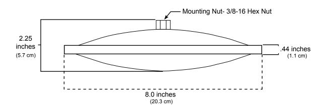
**AW339 Specifications:** • Continuous power handling: 135 watts • Impedance: 4 ohms • Overload Protection: Polyswitch • Frequency Response: 10Hz to 17kHz • Electrical Connecion: 3ft. - 16 guage, 2 wire • Dimensions: 8 in. diam. x 2.25 in. high • Recommended Amplification: 125 - 150 watts at 4 ohms
